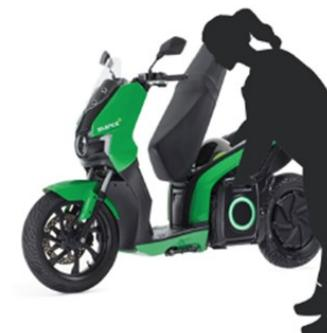
Make sure that the battery is properly secured
