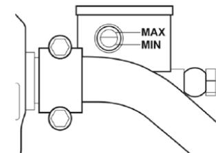
**WARNING:** brake fluid can damage the scooter's paint and plastic parts if spilled.
