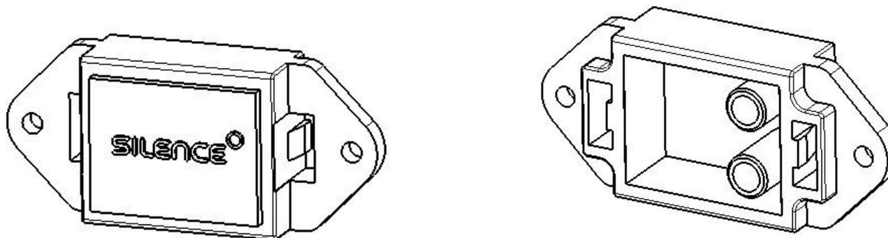
**WARNING: do not put the protective cap on while the scooter is plugged in and never get the connector wet (even with the cap on).**
