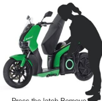
Press the latch Remove the battery pack
