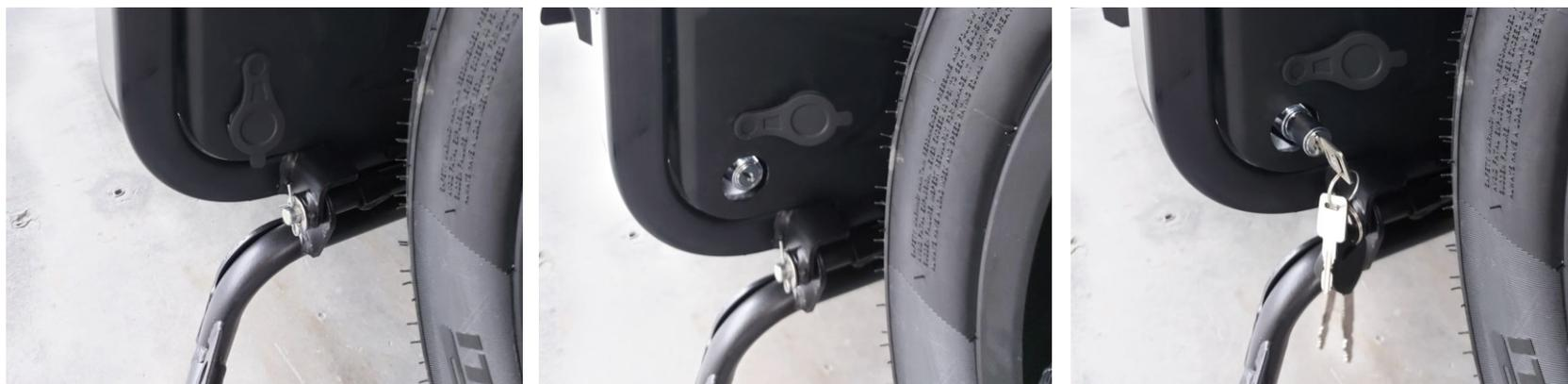
**IMPORTANT:** Never remove or insert the battery pack when the scooter is charging or with the key in the ignition. Make sure **not to unfold the handle before pulling the pack out** (unfold it after the battery has been removed from the scooter).
