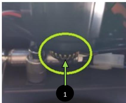
The screw is accessed from the two openings on both sides of the front fender. The adjustment screw is in a place that is not easy to access; if you cannot manage to adjust it yourself, please take the scooter to your nearest SILENCE Official Service Centre.
