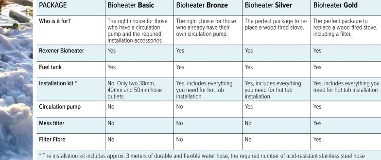
\* The installation kit includes approx. 3 meters of durable and flexible water hose, the required number of acid-resistant stainless steel hose clamps and connectors for the hot tub's outlets. Included connectors for hose sizes: 50mm and 75mm, 2 T-pieces and sealing tape. With the installation kit, Rexener Bioheater is in principle suitable for all the hot tubs on the market.
